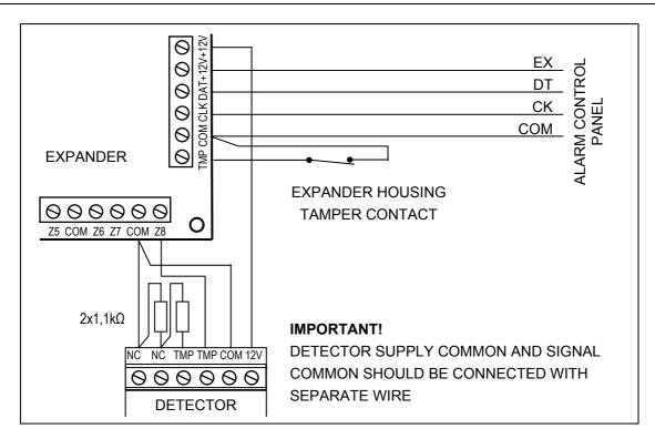
Fig. 13. Connection of 2EOL detector to expander when there is small distance between the control panel and the expander (the detector is distant from the expander).
