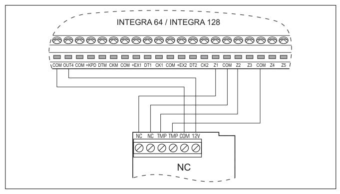
Fig. 9. Example of connecting NC type detector to control panel (NO type detector is to be connected in the same way).
