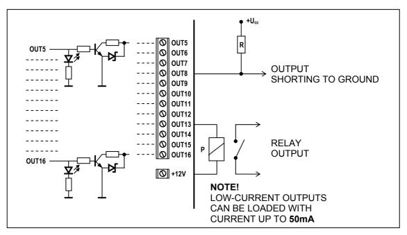
Fig. 15. Connection of loads to low-current outputs (OUT5..OUT16) and signals from these outputs (e.g. to radio messaging transmitter).
