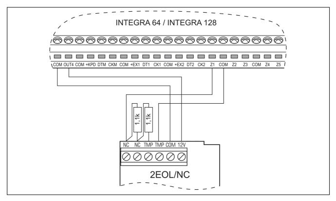
Fig. 12. Example of connecting NC type detector in 2EOL configuration to control panel (NO type detector is to be connected in the same way).
