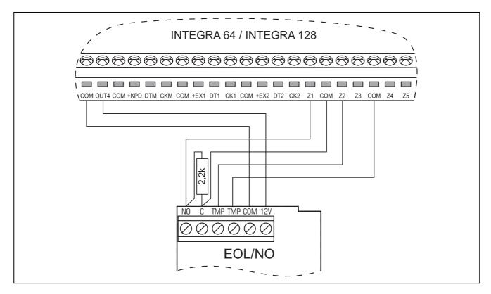
Fig. 10. Example of connecting NO type detector in EOL configuration to control panel.
