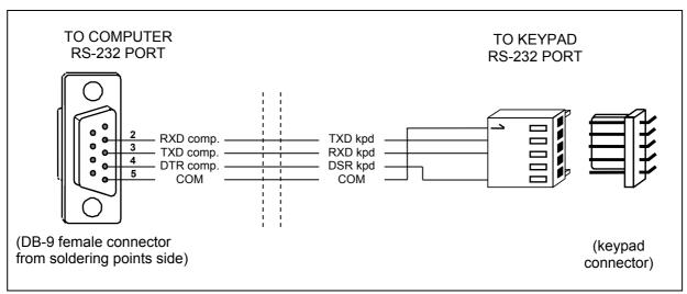
Fig. 6. Connecting computer to LCD keypad RS-232 port.
