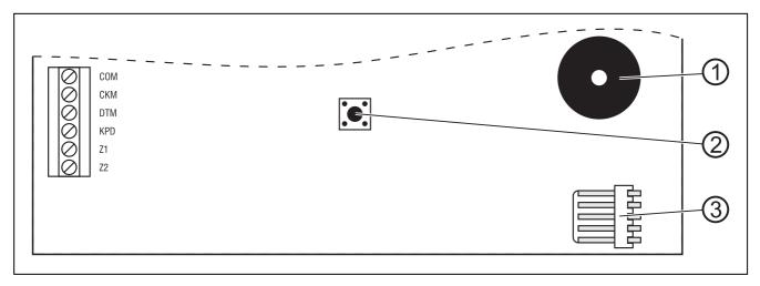
Fig. 2. Partial view of keypad board: INT-KLCD-GR / INT-KLCD-BL / INT-KLCDR-GR / INT-KLCDR-BL.
